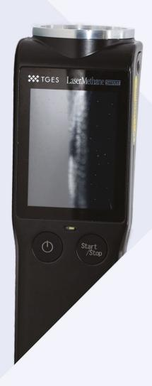
The detector measures the characteristics of methane, which is absorbed into the laser beam (infrared beams) of a specific wavelength (infrared absorption technology). The directed laser reflects back a diffused beam from the target, where the device will receive the reflected beam and measure the absorptivity of the beam, that is then calculated into methane column density (ppm-m).
